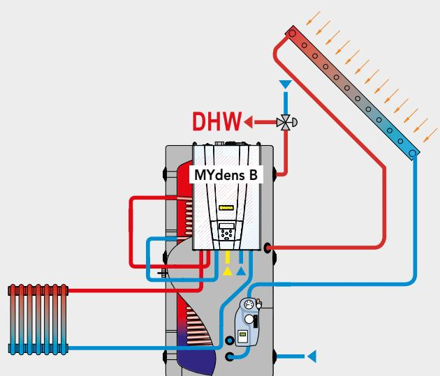
**MYdens** can be backpacked together with a double coil boiler with electronic anode protection as standard, creating an autonomous DHW producer that can be connected to a solar system. It is the ideal solution where there are high peak demands for hot water and heating. It does not require a thermal power plant.
