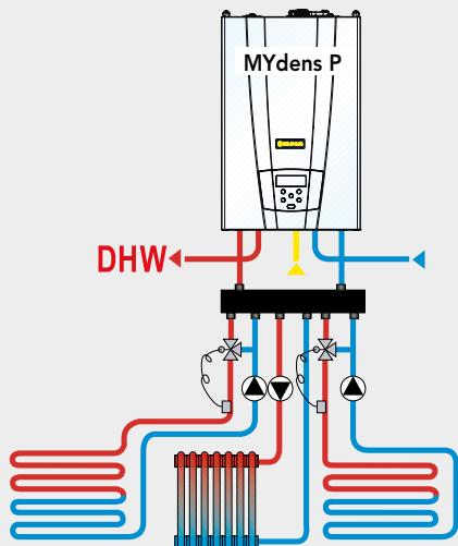
**MYdens**, in combination with the S.I.M. D hydraulic unit, complete with low loss header, can manage up to 3 heating circuits at the same time. Dialogue with boiler and outdoor temperature sensor allows sliding temperature operation.
