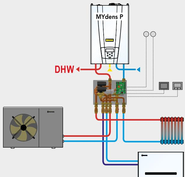
**MYdens** can be included in the 'Factory-Made' ECOhybrid system; with the heat pump connected, system efficiency and energy savings are optimised.
